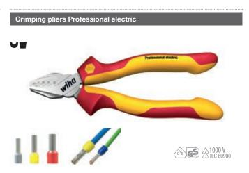
Meets your requirements: Safe pressing in marked trapezoidal/ semi-circular profiles. Lowers your costs: Durable thanks to highquality, chromed plier surface to prevent corrosion. Offers you full protection: Each tool individually tested at 10,000 V AC and approved for 1,000 V AC.
